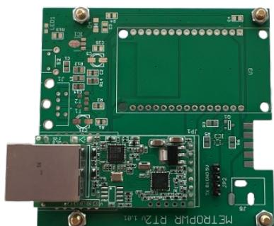
**Note:** Before ordering the FXLAN board, check that your Wattmeter has the **JP2 connector** installed.
