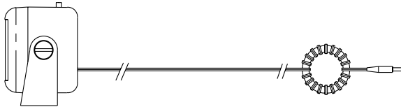
Figure 8. Power lead suppression with ferrite fitted
